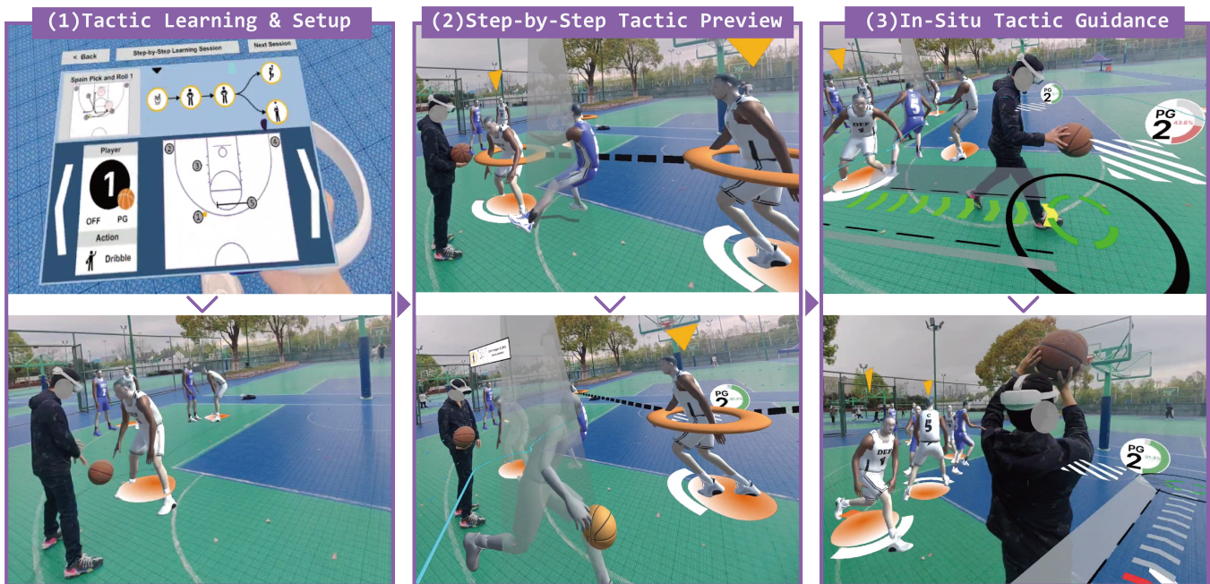
Figure 1: An example usage scenario of VisCourt: (1) Utilizing the navigation view, incorporating a basketball tactic board for supporting tactic learning and setup. (2) Following the tactic breakdown, players engage in a step-by-step tactic preview with a ghost. (3) Employing a set of in-situ tactic guidance both on the court or on players aids to execute the tactic.
